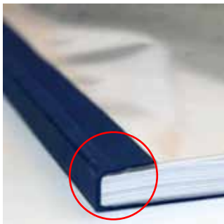
Thermal Binding: tape or binding material wrapped on spine and heat sealed
